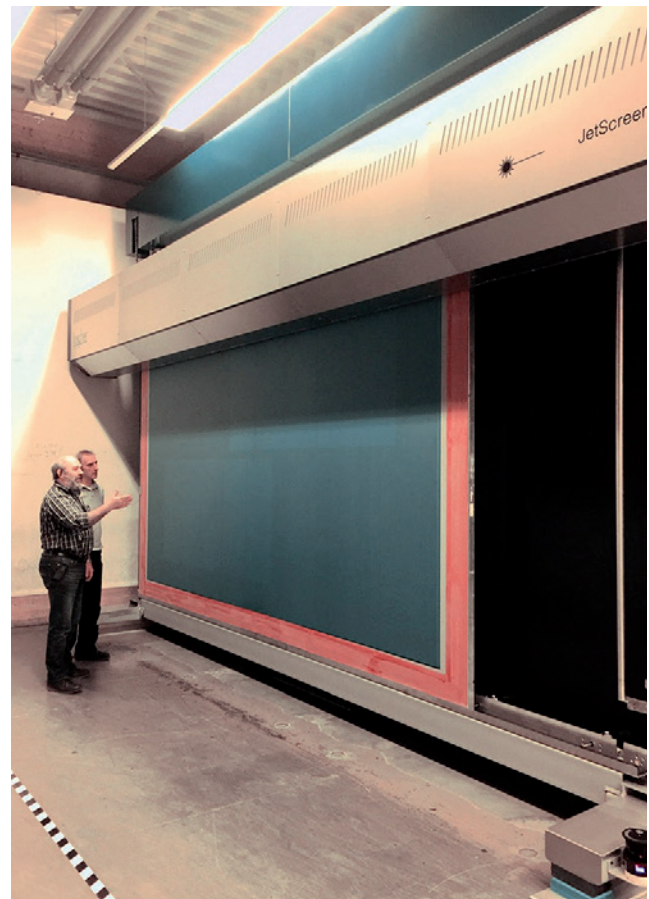
The newly installed XXL JetScreen! LT 55/32 at Joh. Sprinz's Grünkraut plant
