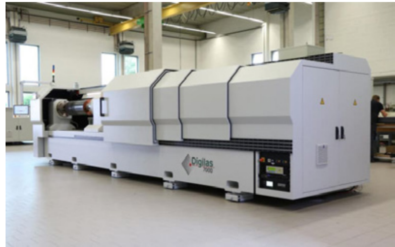
The Digilas from Schepers for direct engraving of gravure and embossing cylinders
