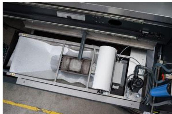
*Water tank with automatic belt filter*
