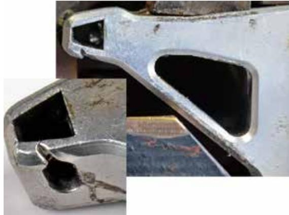
*It is easy to see the groove cut into the stylus arm by years of engraving.*
