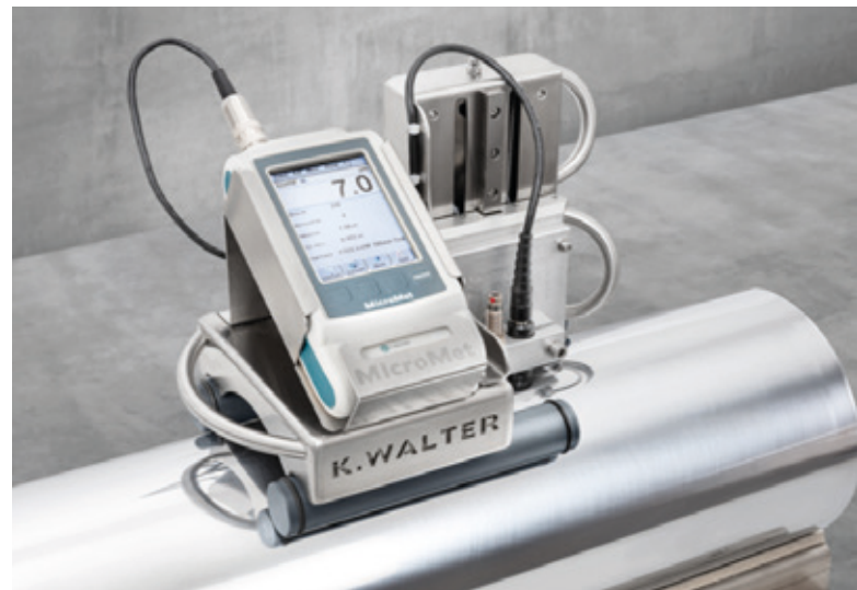
Precise coating thickness measurement now also on chromium(III)
